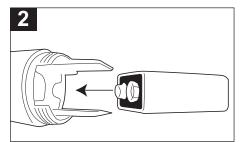
Insert one 9V battery, making sure to observe the correct polarity (+/–). Twist the battery cover clockwise to put it back on.
